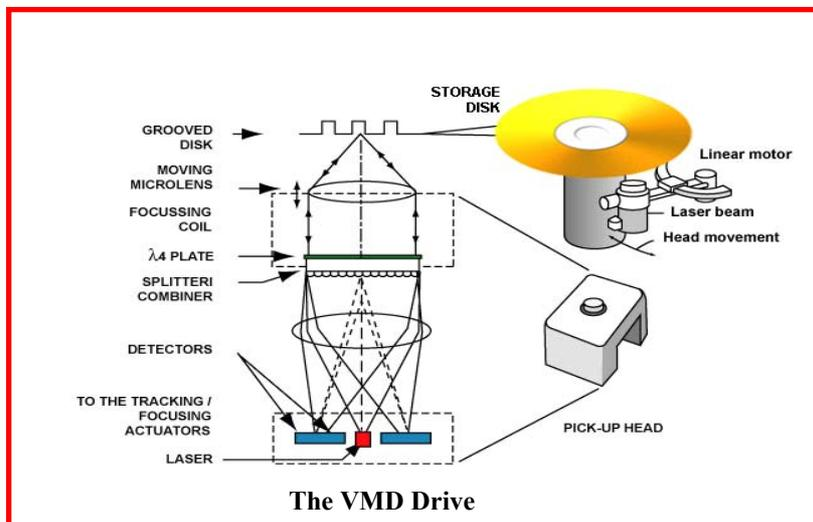
**Pick-Up Head:** Another vital component of the VMD player is the Optical Head (*pick-up*) that includes lasers, mobile actuators and lenses for picking up the reflected laser beam and passing it over to a multifaceted photodiode receptor which receives the signal from the VMD disc. VMD players require high quality optical *pick-ups*. Not all DVD *pick-ups* can be used for VMD player.
